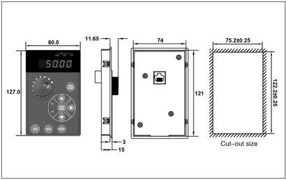
S3100 supporting box of extending keypad external dimensions and mounting hole size
