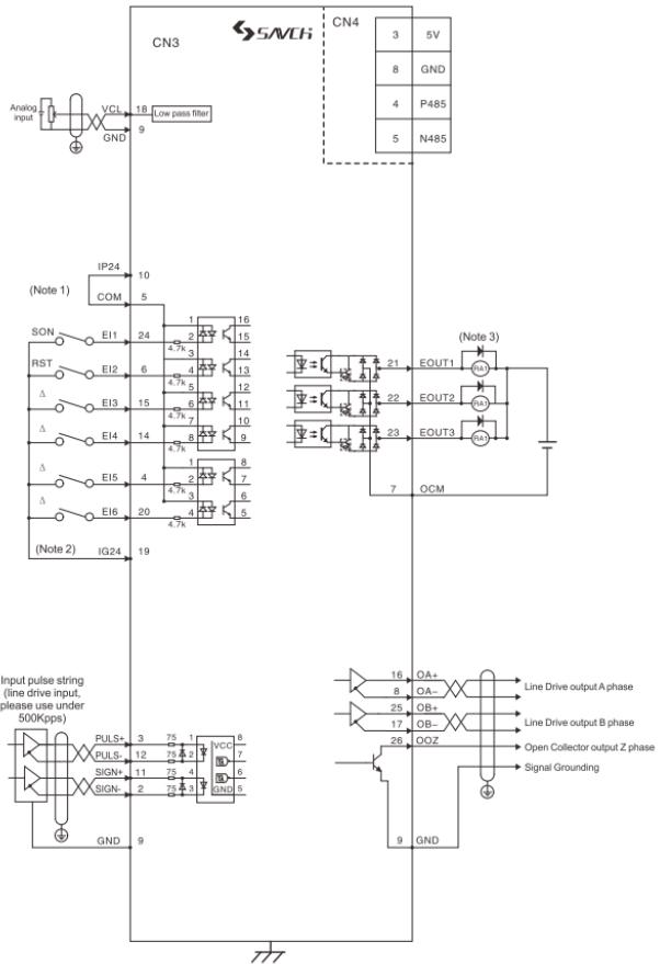
**Note 1:** When the external power are adopted, do not connect the COM with IP24, external power supply 24V connected to COM.
