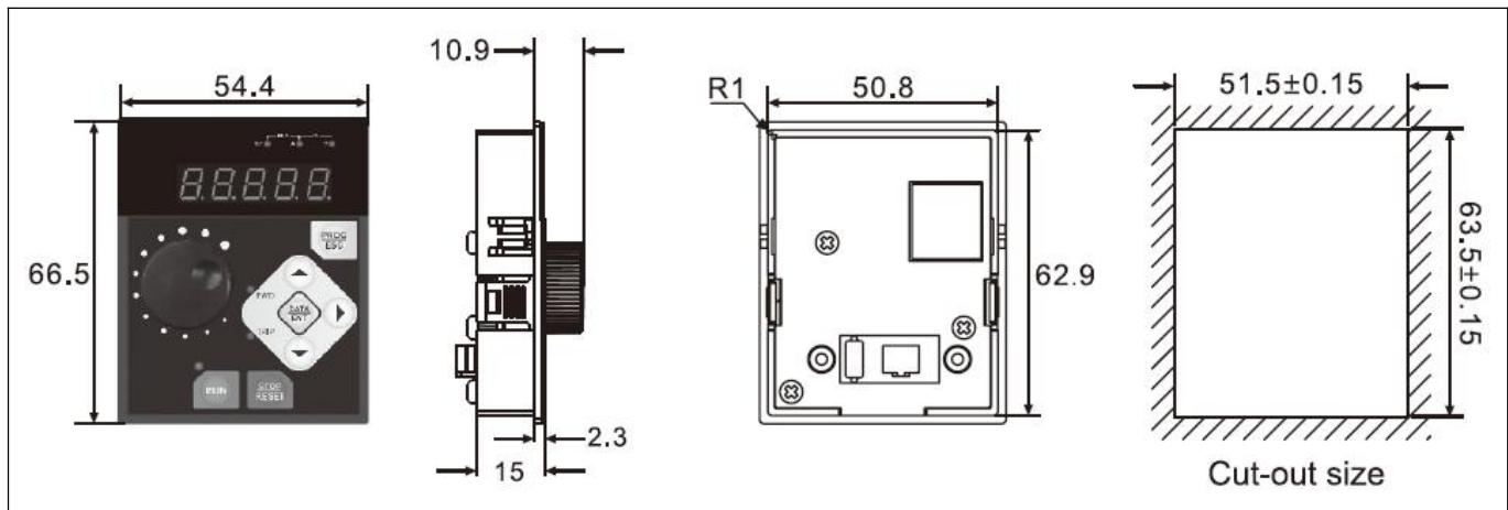
Remote keypad (EL-OP-A2) external dimensions and installation dimensions.
